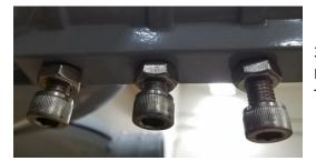
3 c) – Mounting bolts. DO NOT OVER TIGHTEN
