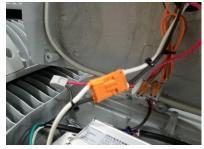
3 a) a. - Disconnect quick connection first from access panel
